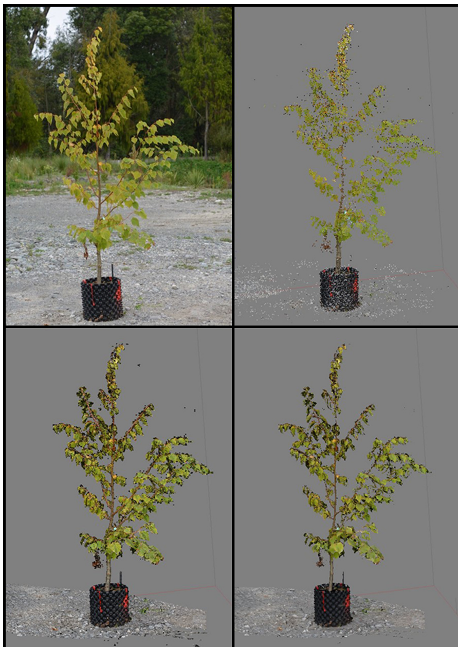
Fig. 2. The four stages of model generation: (top left) the original photo; (top right) the sparse point cloud model following SfM photo alignment; (bottom left) the dense point cloud following MVS; (bottom right) mesh model. Each point in the model represents a pixel in the original photo. Dense cloud models contain several million points.
